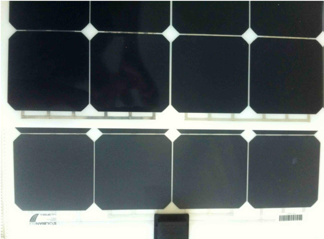
The lower section has been exposed to normal conditions in Pittwater (Sydney) for 12 months. The top section is the same panel after polishing.
